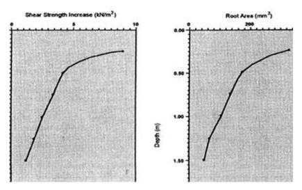
Figure 3: Shear strength of vetiver roots
