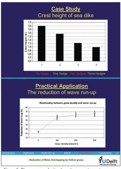
Figure 5: Wave run up reduction by vetiver rows (upper) wave run up reduction by plant density (lower).
